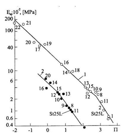
**Notes:** The effect of the stiffness of the stressed-strained state on the wear resistance of materials subjected to hydro- and impact-abrasive wear (a) and a comparison of the coefficients of relative wear resistance of materials exposed to hydroabrasive, impact-abrasive, and cavitation wear
