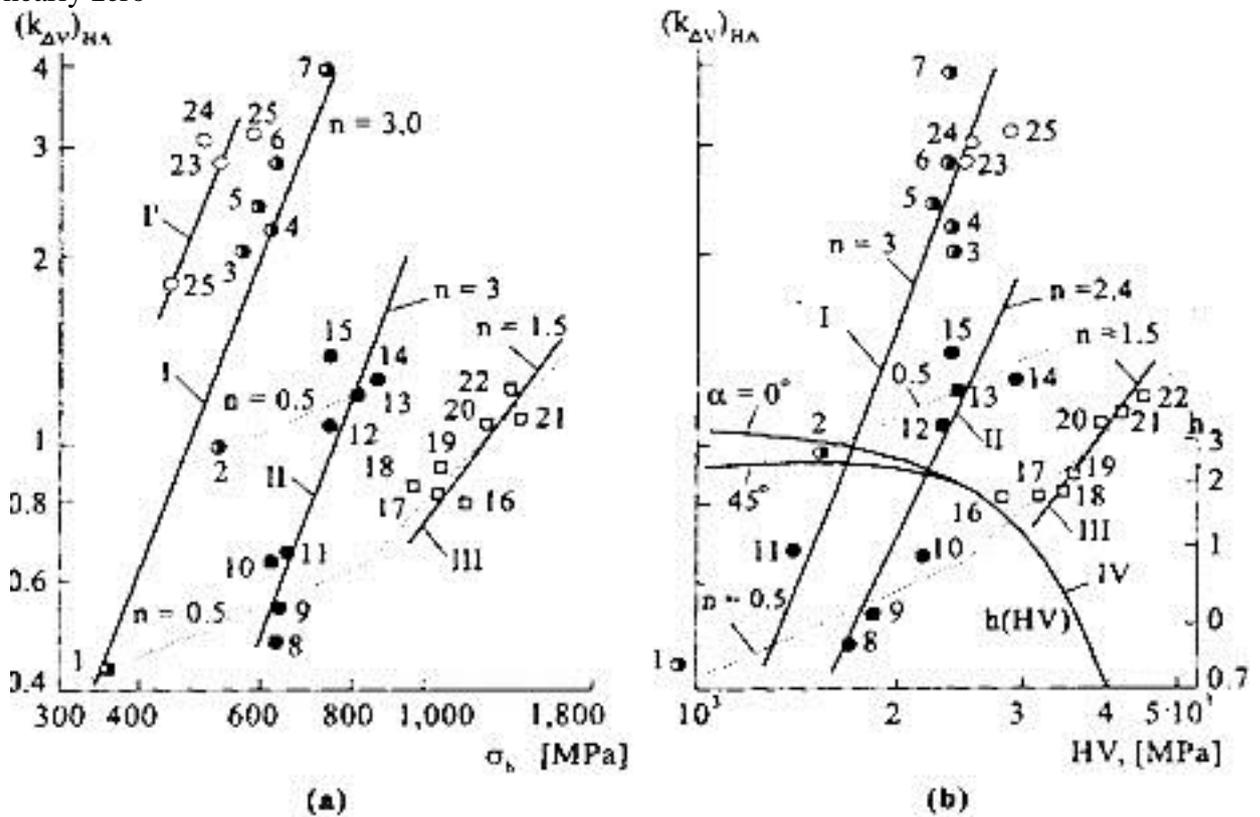
Notes: (a)  $k_{\Delta r_{HA}}$  versus the ultimate strength, (b)  $k_{\Delta r_{HA}}$  versus the Vickers hardness. II(HV) is the dependence of the coefficient of the stiffness of the stressed-strained state of the surface of metals on the hardness for the hydroabrasive flow attacking the wearing surfaces at angles of 45° and nearly zero
